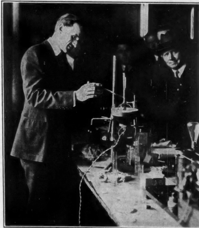
T. S. SLIGH, JR., BUREAU OF STANDARDS, DEMONSTRATING APPARATUS DEVELOPED AT THE BUREAU IN CONNECTION WITH THE COOPERATIVE FUEL RESEARCH FOR EVALUATING THE PERCENTAGE OF DILUTION IN CRANKCASE OIL BY THE TRANSITION METHOD OF VACUUM DISTILLATION
