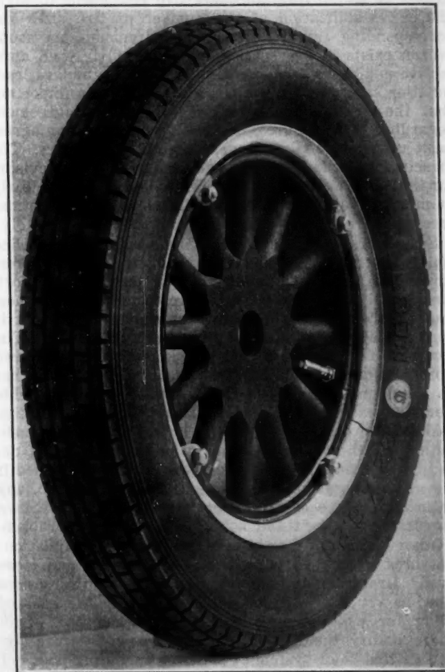
FIG. 8—A COMMERCIAL FLAT OR NATURAL-PROFILE TIRE. This Tire, It Is Claimed, Affords Even Tread-Wear, Easy Steering and Excellent Traction under Practically All Road Conditions
