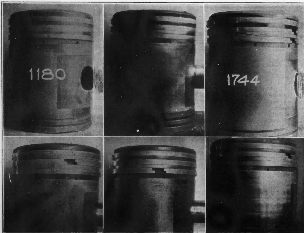
FIG. 6—CONDITION OF THE PISTONS AFTER THE TEST
