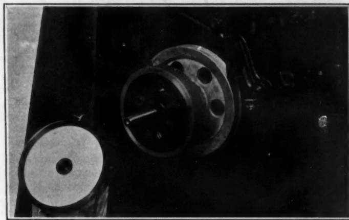
FIG. 6—THE INDICATOR IN PLACE ON THE CRANKSHAFT This Instrument Indicates and Records the Torsional Vibration Occurring in a Crankshaft Operating Normally throughout its Range of Speed and Load. If the Speed is Normal and Torsional Vibration is Absent, the Trace of the White Disc, Which Has Been Removed and Can Be Seen at the Left, Appears as a Circle. Any Torsional Vibration of the Crankshaft and Angular Displacement between the Disc and the Flywheel Cause the End of the Lever Carrying the White Disc To Move In and Out while Rotating. This Makes the Trace of the White Disc Stand Out as a Wave Curve Departing from a True Circle in Proportion to the Intensity and the Frequency of Vibration
