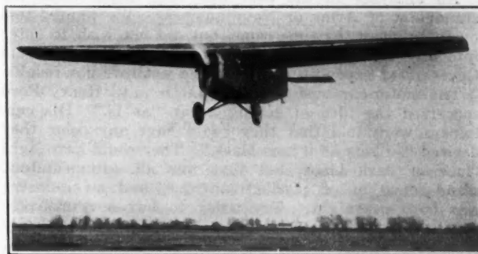
FIG. 1—THE ORIGINAL MAIDEN DETROIT IN THE AIR Carrying 2700 Lb. of Ammunition for the Army, the Round-Trip from Detroit to Oscoda, 150 Miles, Was Made in 3 Hr.
