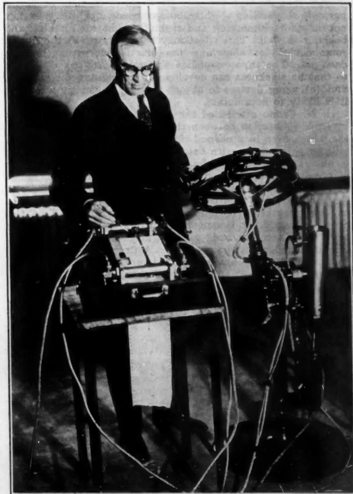
F. F. CHANDLER DEMONSTRATING THE INSTRUMENTS FOR RECORDING WHEEL AND DRAG-LINK MOVEMENT DESCRIBED IN HIS PAPER
